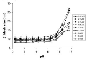
Figure 1. Hydrogel network mesh size for 9 different polymer formulations of P(MAA-g-EG). The values for  $\xi$  increase with increasing pH from 7 nm – 28 nm. The apparent pKa of the hydrogel is 5.8-6.0. Samples are identified as mol% PEGDMA 200/wt% monomer.
